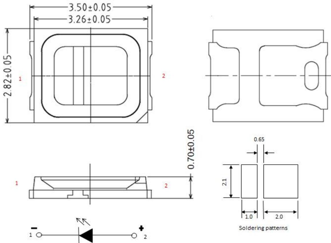
**NOTE:** All dimensions in mm tolerance is  $\pm 0.1$ mm unless otherwise noted.
