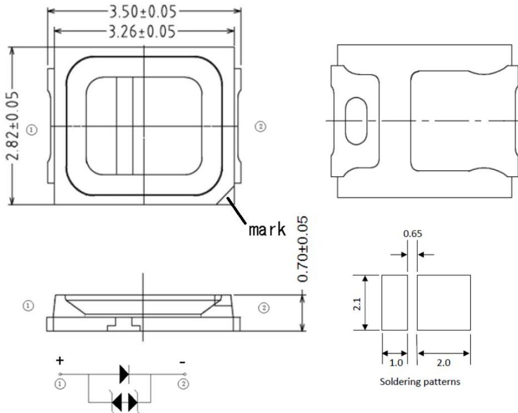
NOTE: All dimensions in mm tolerance is  $\pm 0.1$ mm unless otherwise noted.
